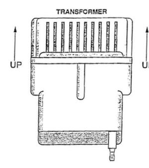
The coil can be checked with a multi-meter, but it is not a definitive test. Since a multi-meter uses only a very small voltage, it can only indicate established traces to ground or complete "open" conditions in the winding.
